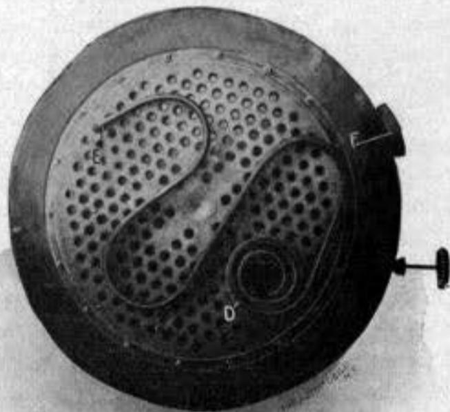
FIG. 4. VAPORIZING COIL IN POSITION.
