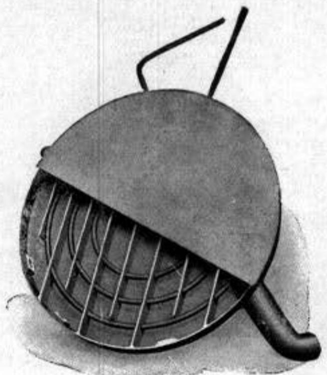
FIG. 6. THE MUFFLER.
